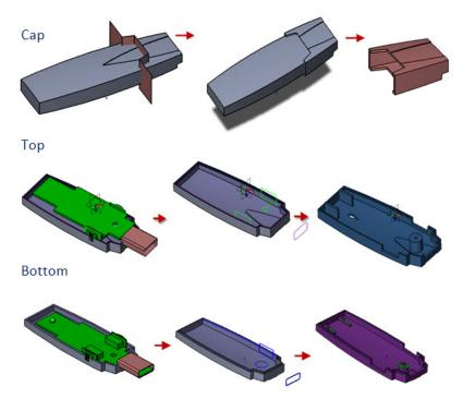
5. As shown above the Base is made up of the Top, Bottom and Electronics
