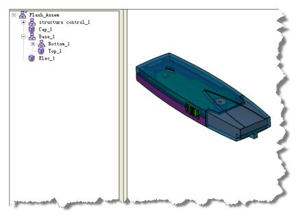
The design of the **Flash disk** is complete. The main product form and fit is defined by the **Structure Control**. Product dimension modifications will directly affect its sub-components. Meanwhile, the established relationship between **Top** & **Bottom** components and **PCB** board ensure that changes in the **Structure Control** are passed along to all sub-components.
