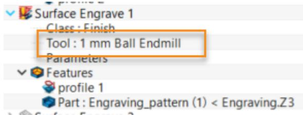
Figure150 Create tool path on the design pattern example step3
